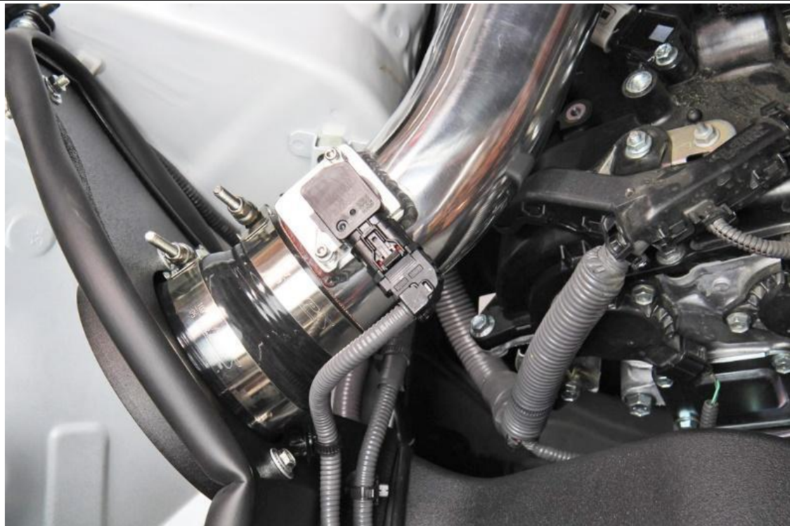
24. Reconnect the mass air flow sensor harness connector.
