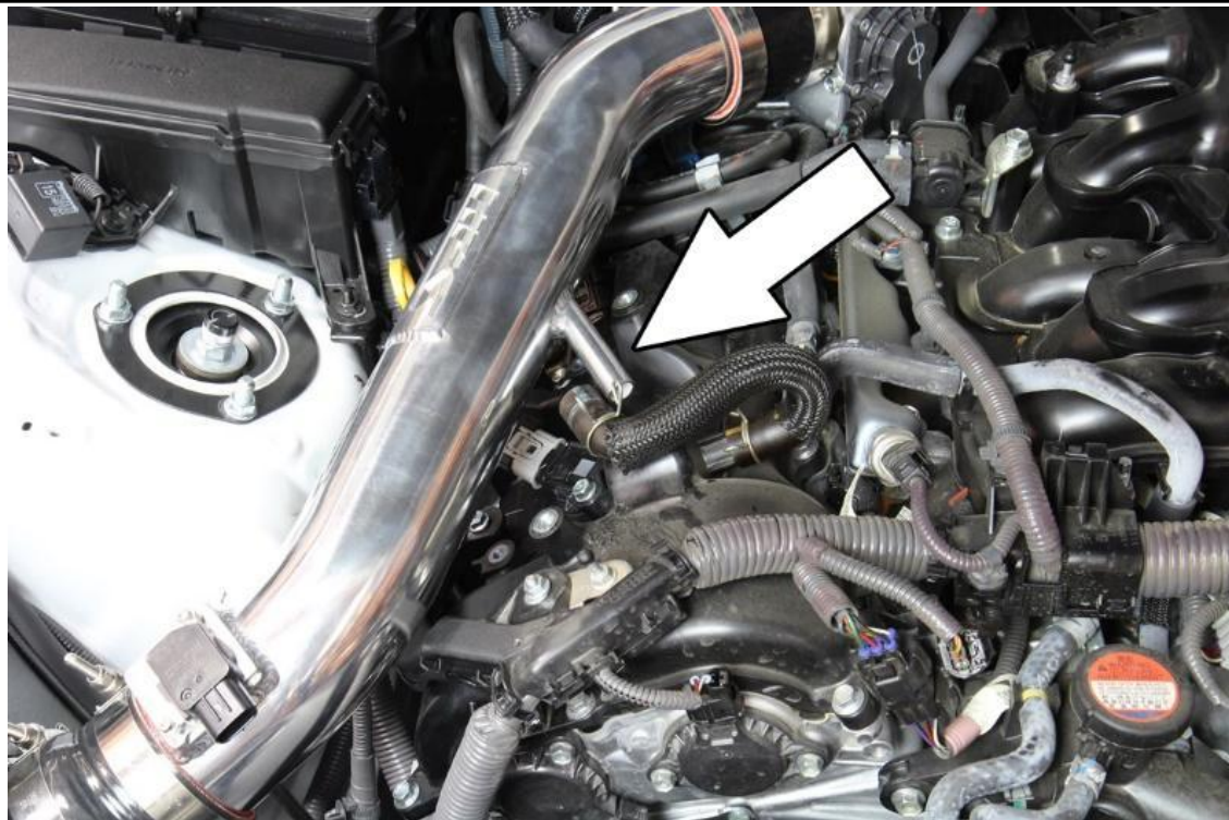
23. Re-insert the crank case breather hose onto the HPS intake barb.
