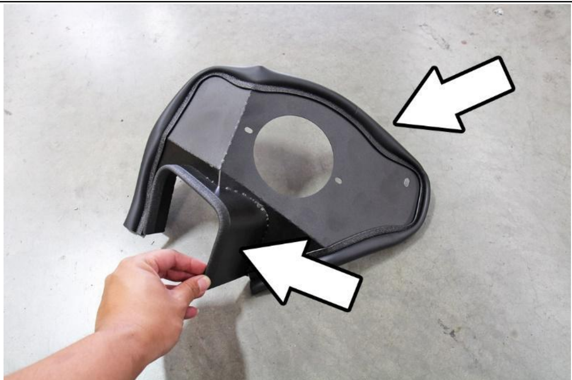
17. Install the thin edge trim onto the air duct opening of the heatshield and the bubble edge trim onto the outer edge of the heatshield.
